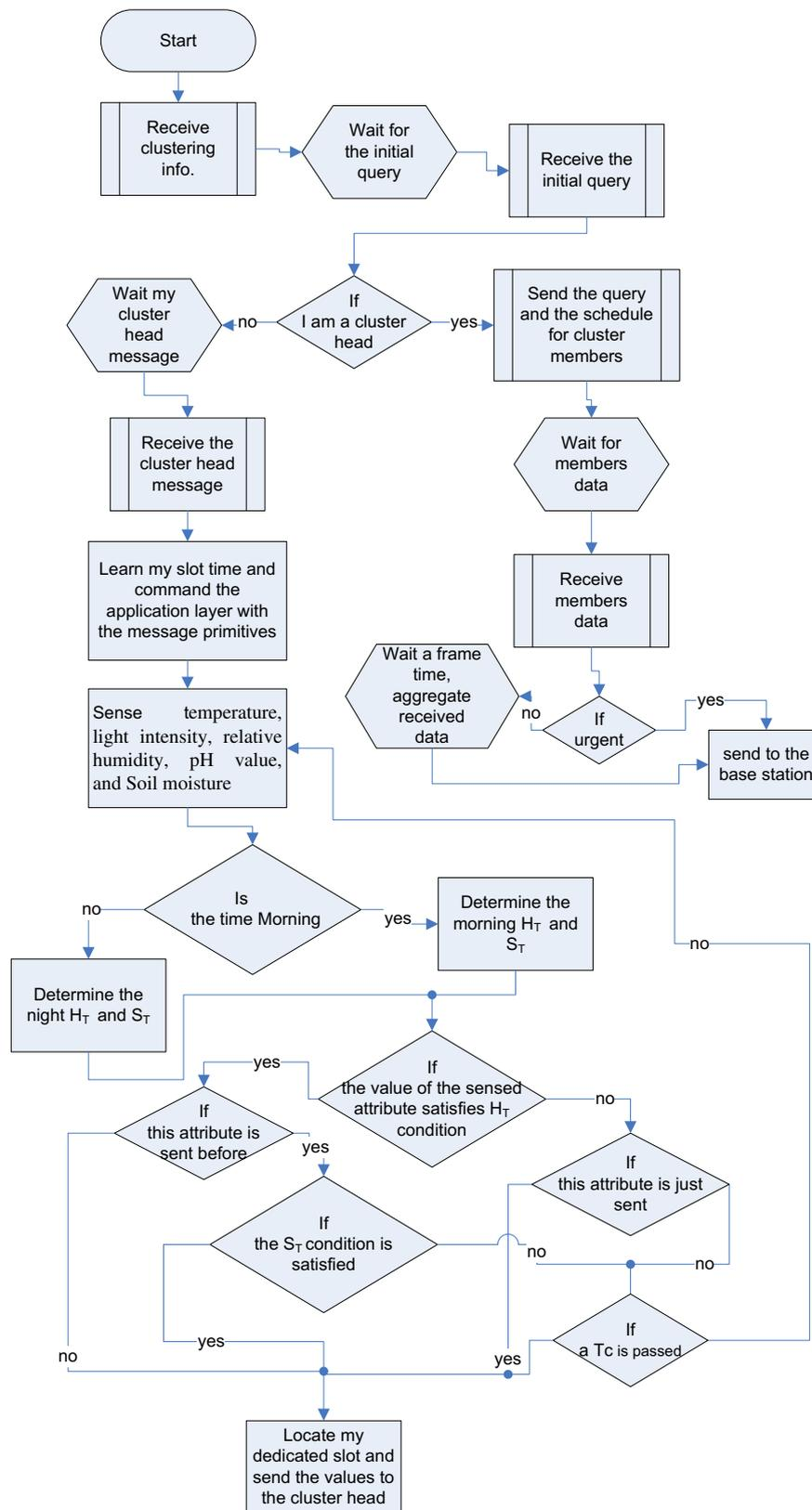
Figure 9 Sensor node procedures.
