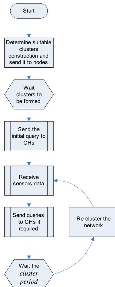
Figure 8 Base station procedures.
